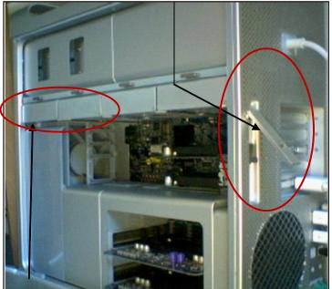
Remove drive sleds 1 and 2. Sleds are marked on the upper right hand side front, 1 being the closest to front of machine. Lay system on its side (side opposite you), this makes screw removal easier, and is necessary for removing the frovnt fan.
