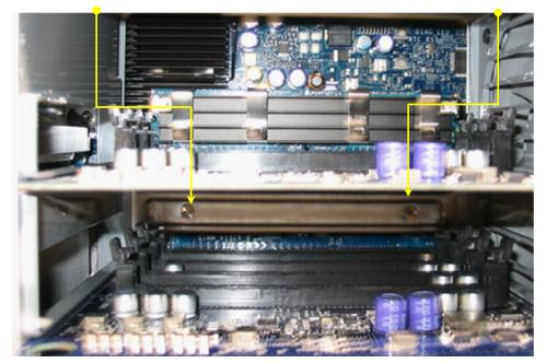
6 - Two screws are located on what would be the bottom of the machine, closest to the case door, were it upright. These must be removed as well.
