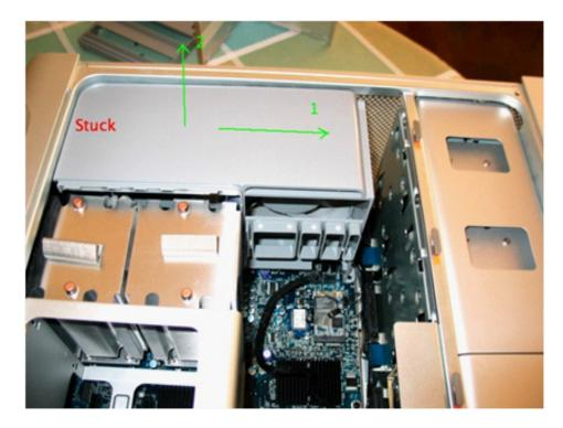
9 - Once front fan is removed, access to SATA ports is revealed.
