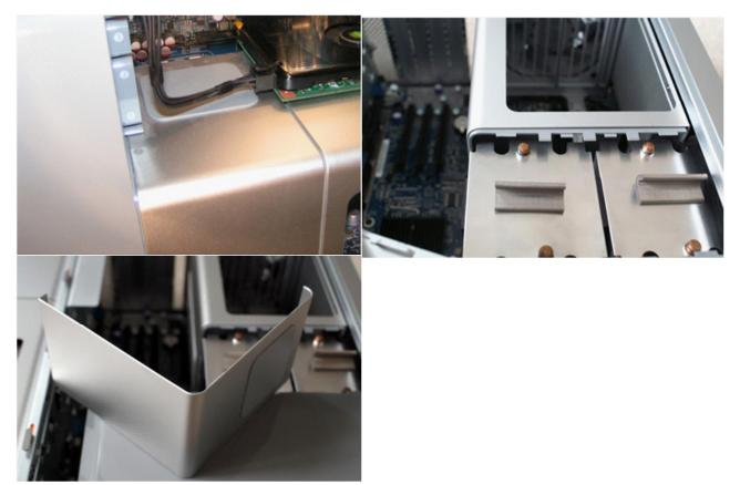
8 - When heat sink cover is removed front fan can now be removed. Grasp top (closest to optical drives and slide PCI cover plate between fan and case. The cover plate will help to separate fan from case. Lift straight up while prying away from case, either front or bottom.
