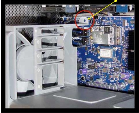
**3** - Remove video card: Begin by unscrewing two large screws on plate holding cards in. When loosened, remove plate, then video card.
