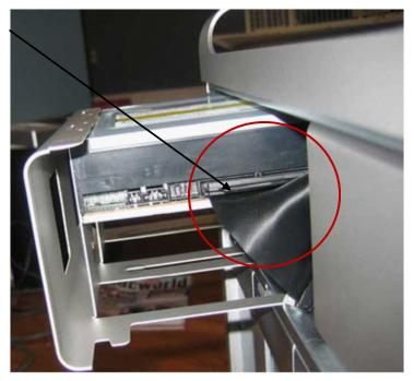
12 - Using a straightened paperclip, eject tray and pull out until completely out. Remove bezel from Blu-ray drive. This can be done by locating three bumps holding bezel in place and carefully lift edges over bumps and sliding bezel up.
