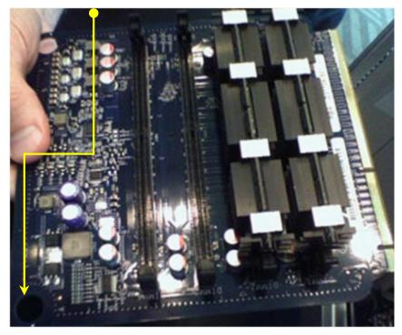
5 - Remove two screws at bottom of memory bay.
