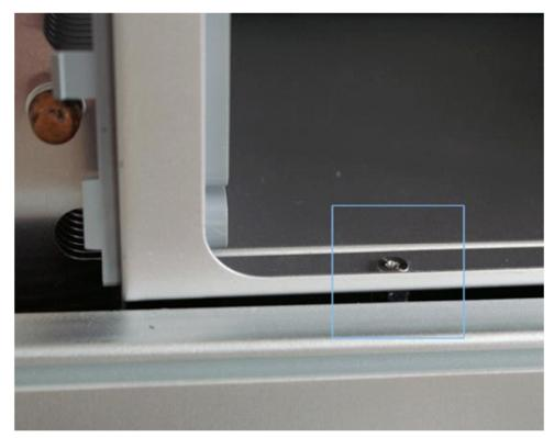
Once screws have been removed, the memory bay should be movable. It is not removable, but there is play and wiggle room. Rock bay towards back of system (where USB ports, fire wire ports, and video card output is) to loosen the heat sink cover. Heat sink cover will have to be rocked and shifted left/right as well.
